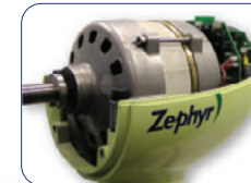
New Power Generator and Control Board
